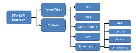
Figure 6: Diagram showing all the electrical components of the robot
