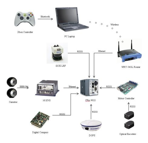
Figure 3: Diagram showing all the hardware components of the Q system and how they are integrated.
